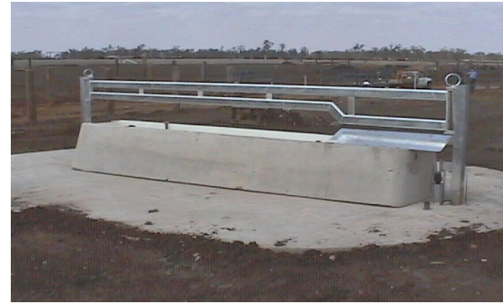
Trapeze-shaped water trough centrally placed on an oval-shaped concrete apron.
