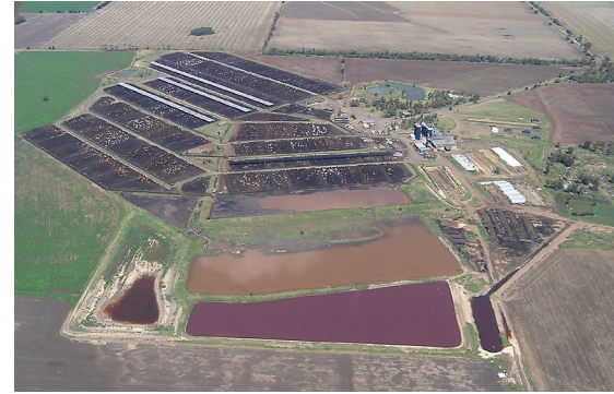
Aerial photo of a feedlot catchment area draining down to a holding pond.
