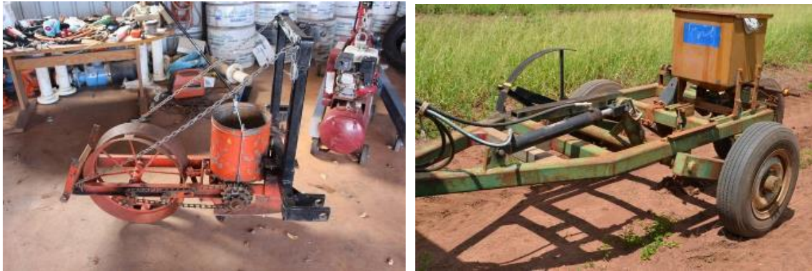
Fig. 5 Planters used for the first and second rounds sowing at Pinnarendi; a. three-point linkage mounted disc opener (first round sowing), b. heavy-duty towed basalt planter (second round sowing).
