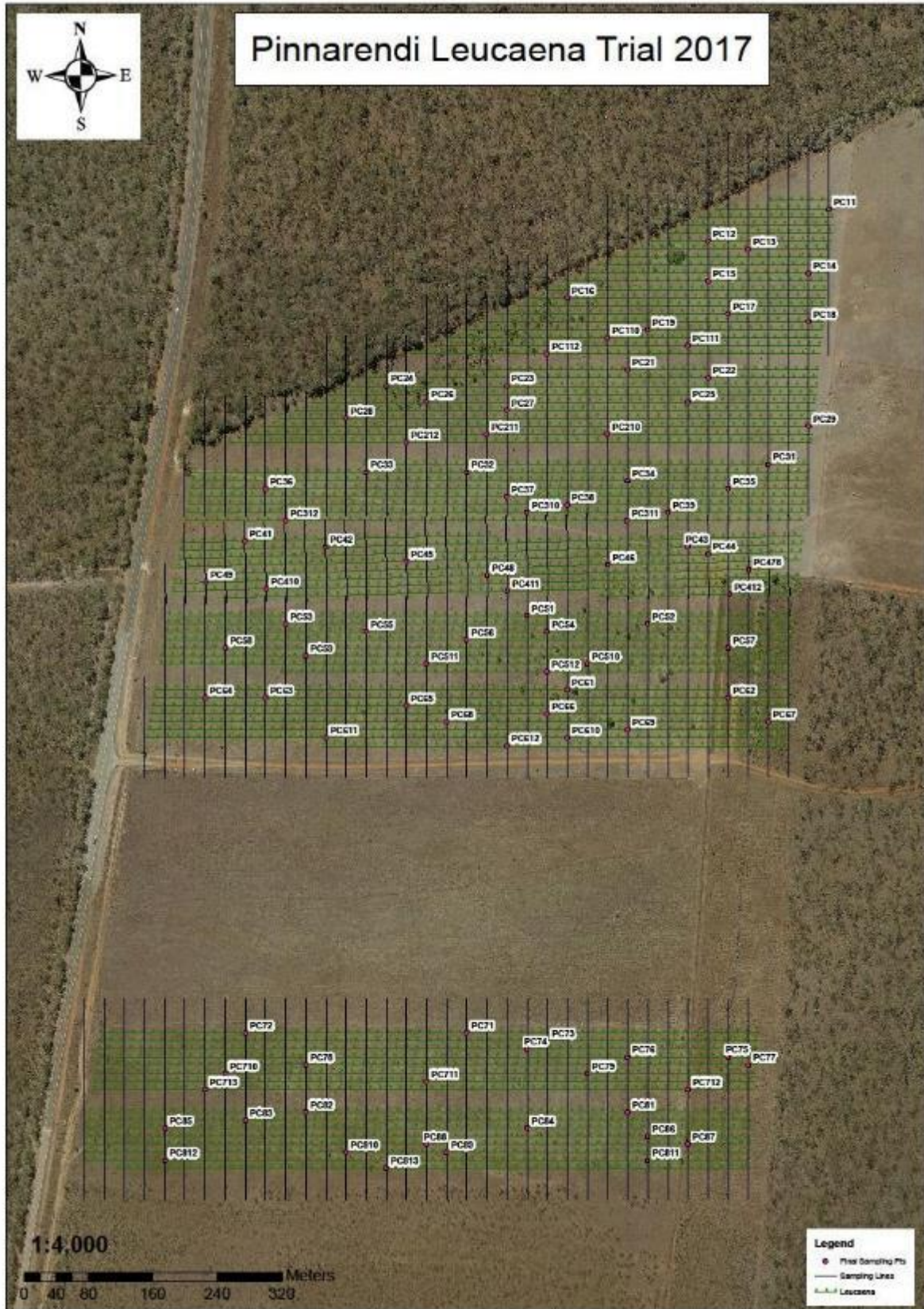
Fig. 10 Start locations of sampling plots (98 plots in total) for leucaena population and height survey based on row number with 25 m grid overlay.
