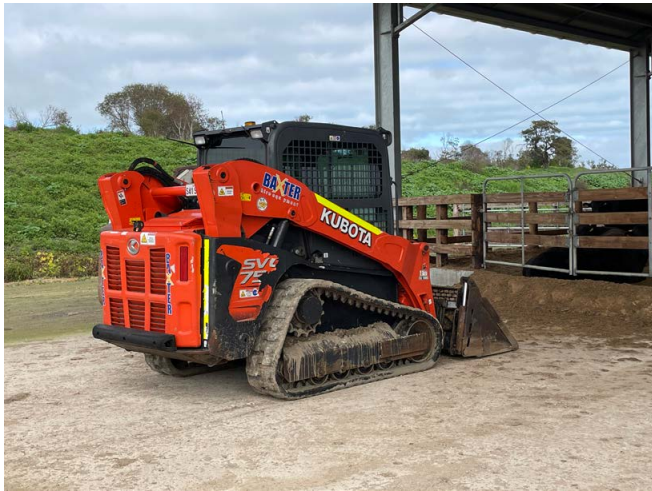
Photograph 55: A tracked skid-steer is ideal for cleaning smaller pens
