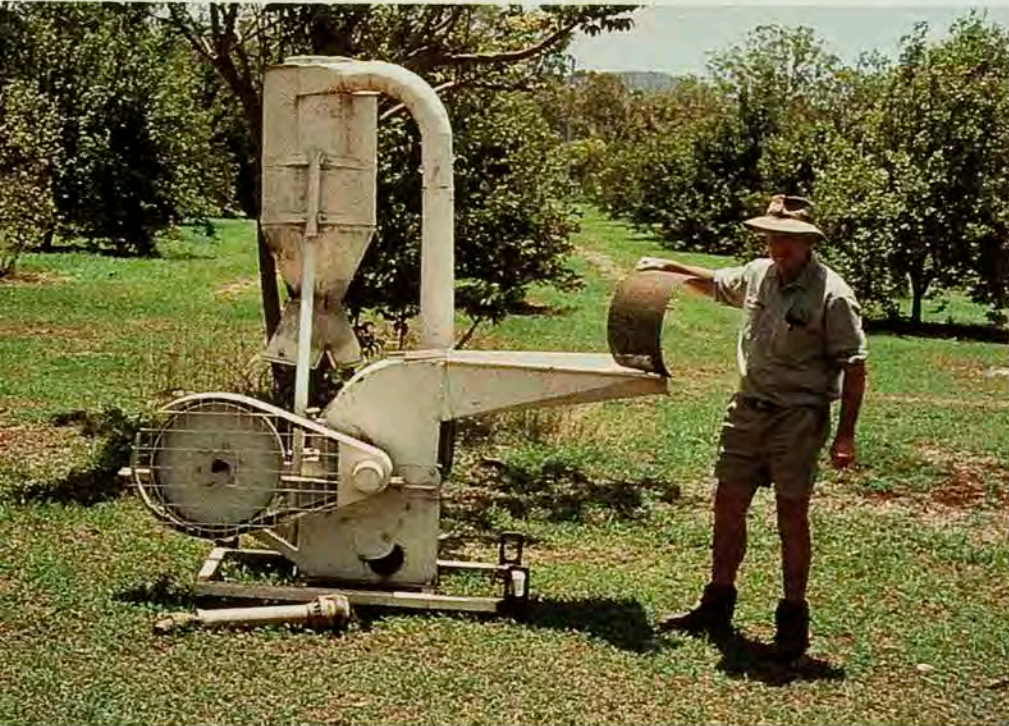
Dr John Hopkinson developed this modified hammer-mill to speed up treatment of hard stylo seed.
