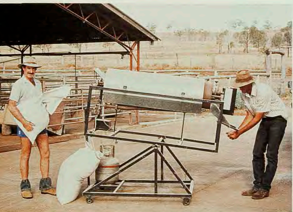
Col Paton found this revolving heated cylinder gives the best results with fine stem stylo.
