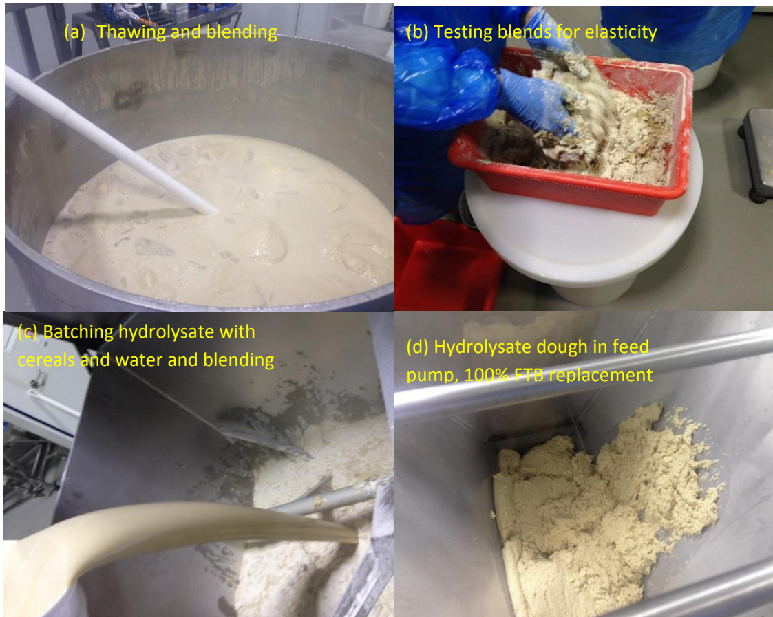
Figure 6 ProForm HMEC trial preparation (a) Blending hydrolysate (b) testing mix elasticity (c) Preparing batches for pumping (d) Pump feed with single batch
