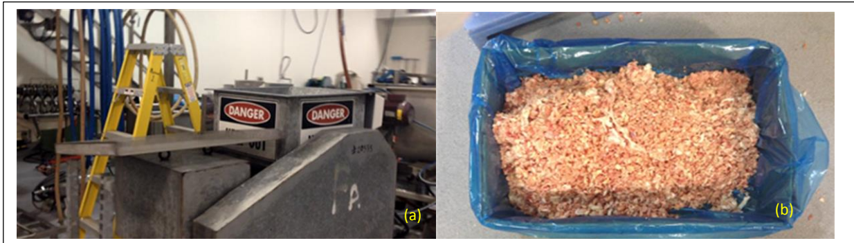
Figure 2 Older style hogger (a) and hogger size reduced bone (b)
