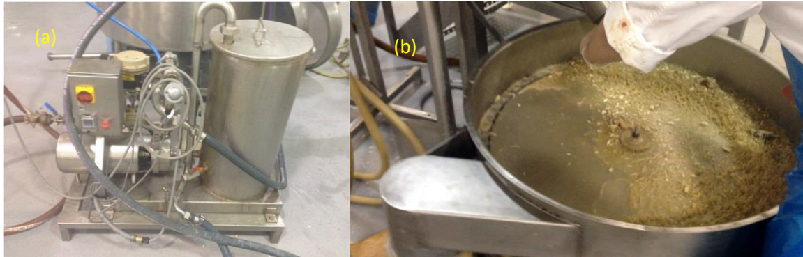
Figure 4 Equipment challenges (a) Holding tank heating (b) Kason screen blinding
