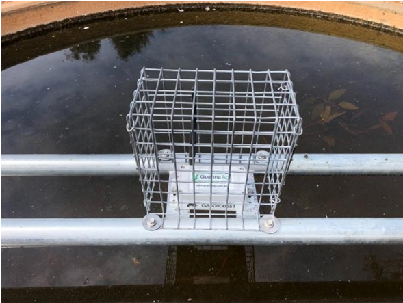
Figure 4: Redbank water trough sensor
