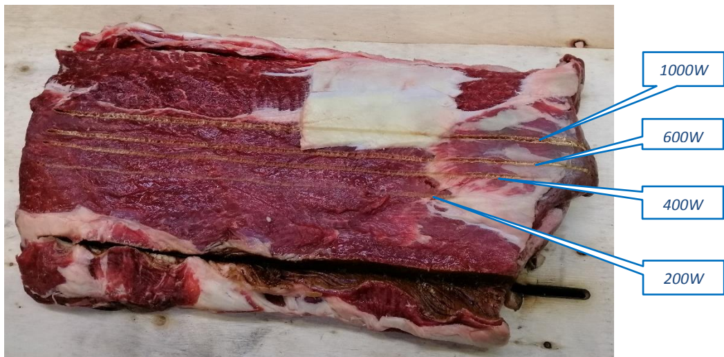
Fig. 8 - Laser engraving marks at different power settings on a section of beef loin
