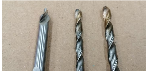
Fig. 4 - Drill bits used for testing. [Left]: centre drill; [Centre]: 4mm drill bit; [Right]: 5mm drill bit
