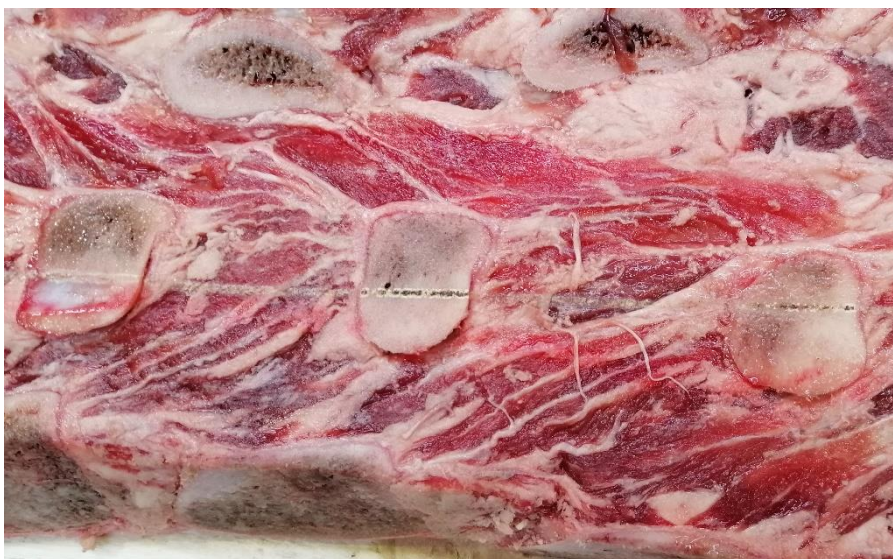
Fig. 9 - Laser engraving on bone at 200W. The line has good contrast against the white bone
