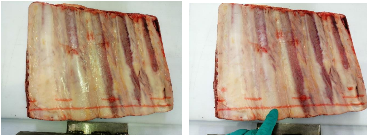
Fig. 15 – Red Ink line, dash and dots sprayed on ribs. [Left]: image captured immediately after applying ink; [Right] image captured after wiping line at two minutes. Ink was dry before two minutes
