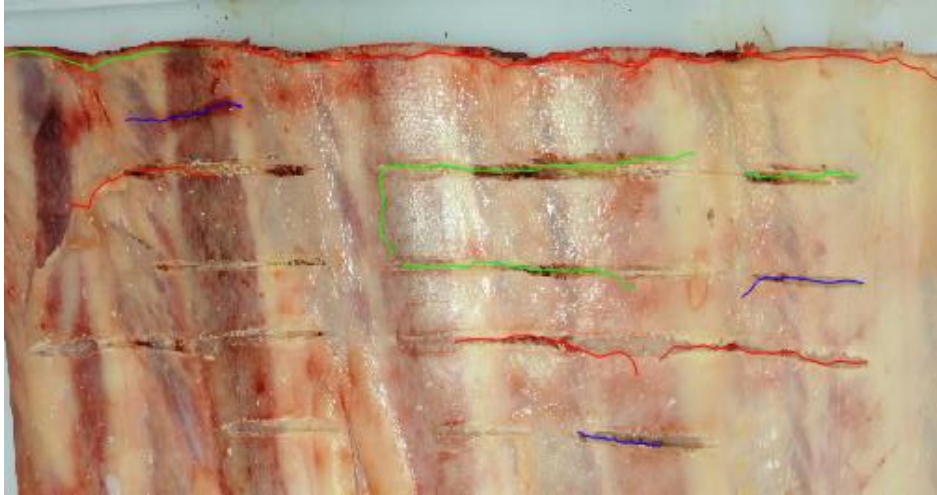
Fig. 22 – Preliminary vision results attempting to detect the rotary scoring lines. Inconsistent widths and intermittent lines were the main reasons for failure
