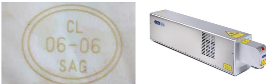
Fig. 6 - Product code produced from Linx laser marking on pig skin (Linx printing technologies, 2019).
