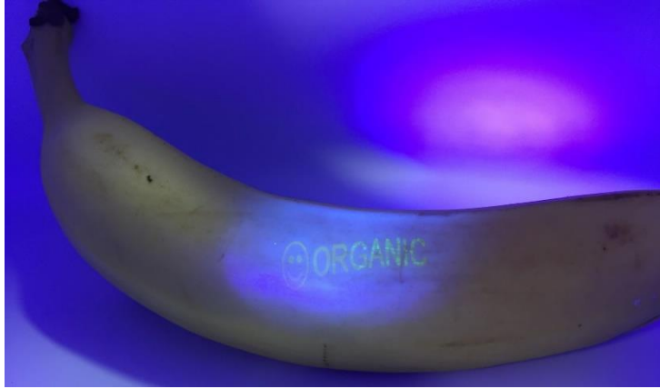
Fig. 13 - POLYtrust® HACCP invisible ink demonstrated on a banana in black light (RPL Regal Packaging Ltd, 2019). This ink is now discontinued.
