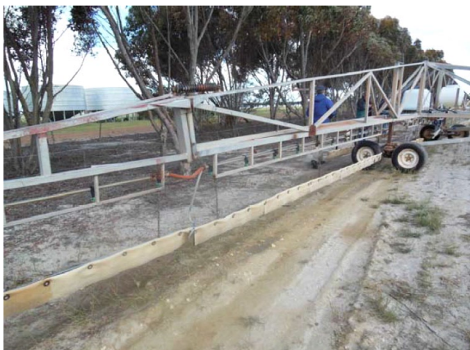
Figure 11. A blanket wiper developed for assistance in controlling weeds in herbicide sensitive crops. The wiper utilises differences in height between the pest weed and the crop.
