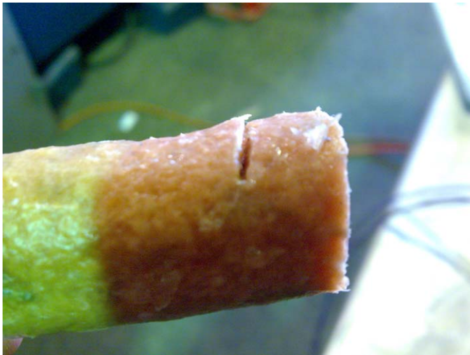
Figure 1. Sausage test result, 4mm deep cut
