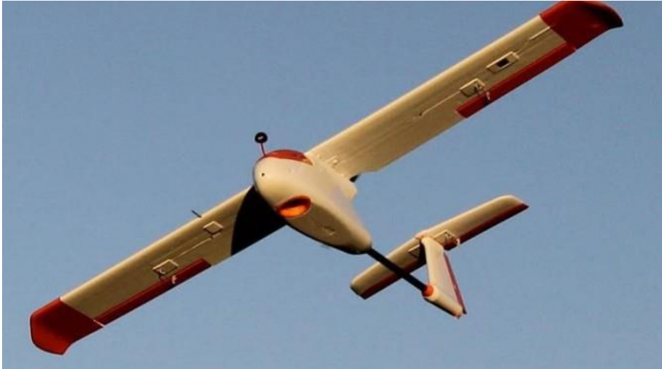
Figure. 2 Goshawk Airframe is a fixed wing RPA used by Hitachi for the initial flight tests
