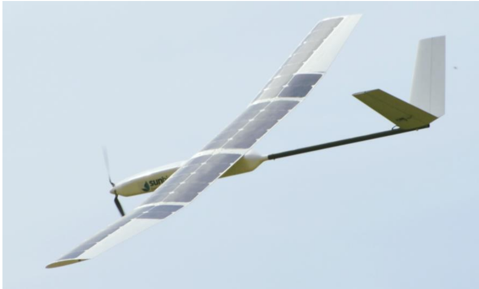
Figure. 4 The fourth airframe used at Calliope Station for Hi-Res imaging (Sunbirds®) with solar panels on its wings to recharge its battery pack for enhanced flight endurance
